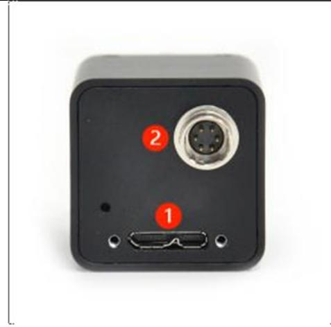
Figure 9-5 SWIR-UMV series Camera design and its ports
