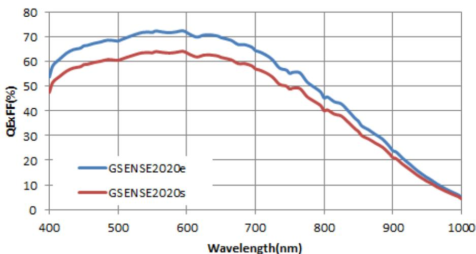
Figure 2-8 MaxCam-2020Me-TE spectral response curve
