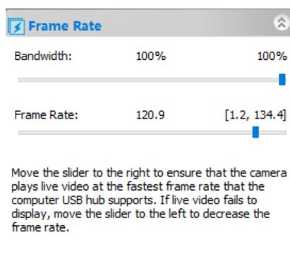
Figure 14-1 Bandwidth and precise frame rate settings
