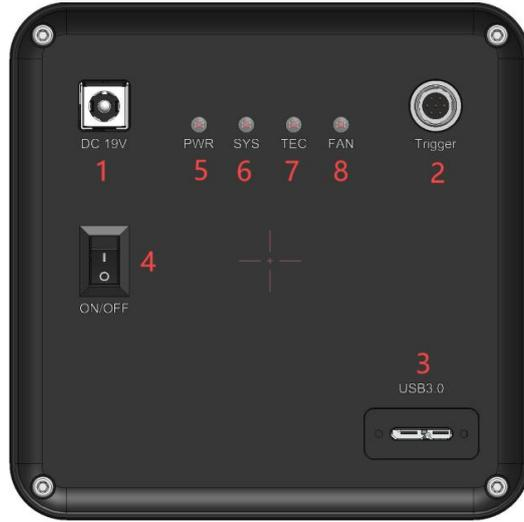
Figure 12-6 MaxCam-811, -411, -461 Camera interface diagram
