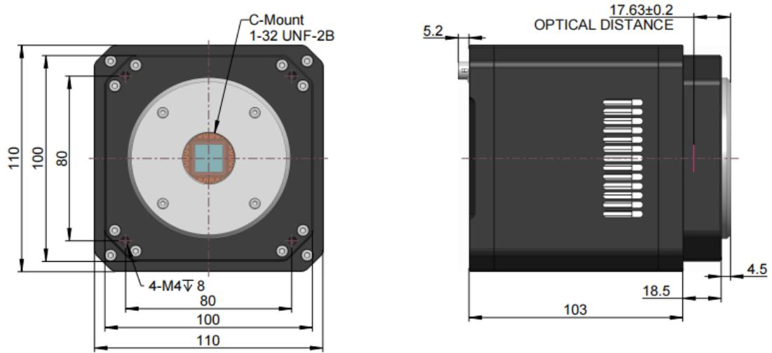
Figure 12-4 MaxCam-2020UV-TE dimensions (mm)
