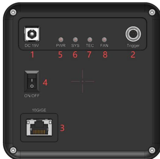
Figure 12-10 MaxCam-811, -411, -461 Camera interface diagram
