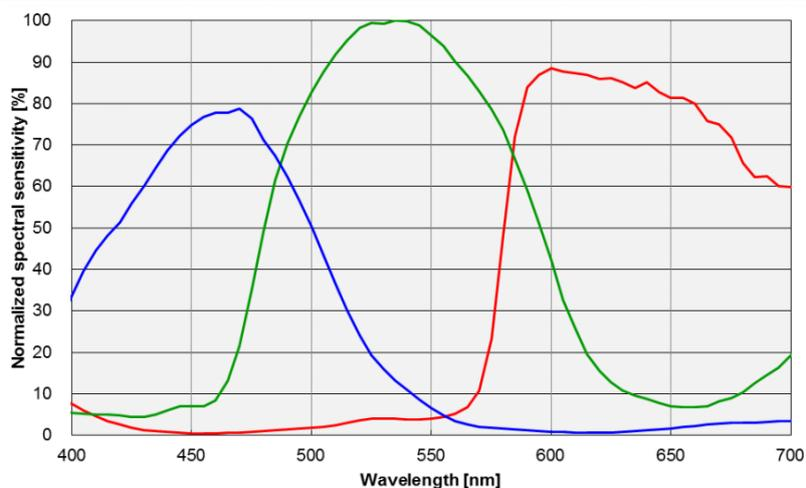
Figure 2-4 MaxCam-461C-TE spectral response curve
