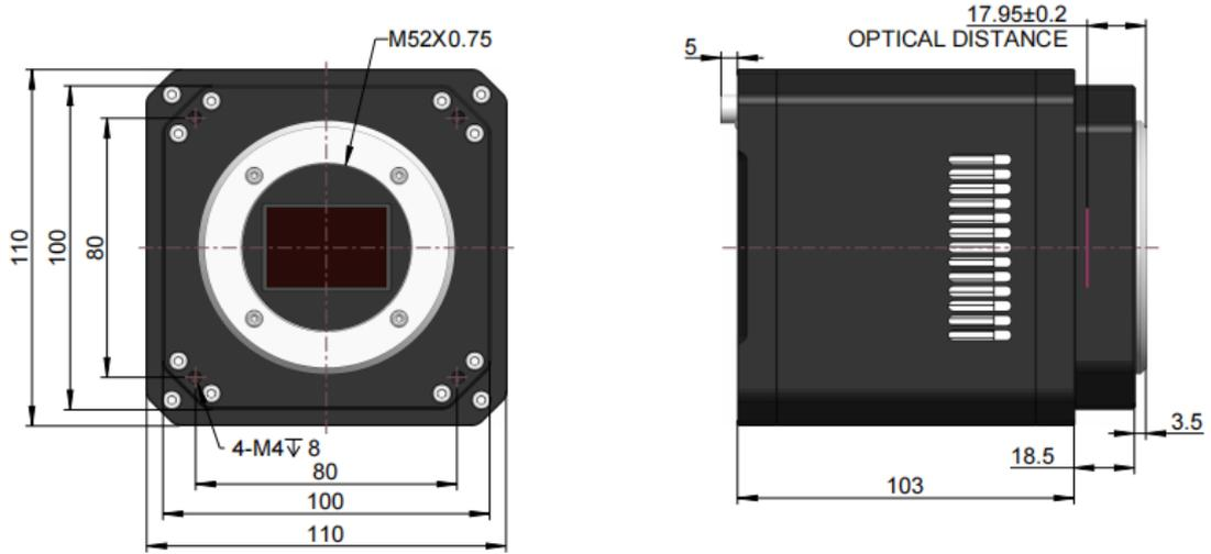
Figure 12-3 MaxCam-455M/C-TE& MaxCam-410C-TR dimensions (mm)
