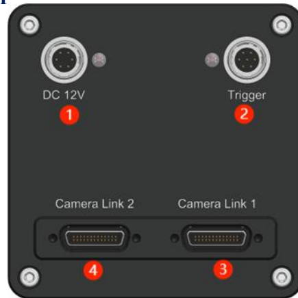
Figure 8- 16 CL interface refrigerated camera
