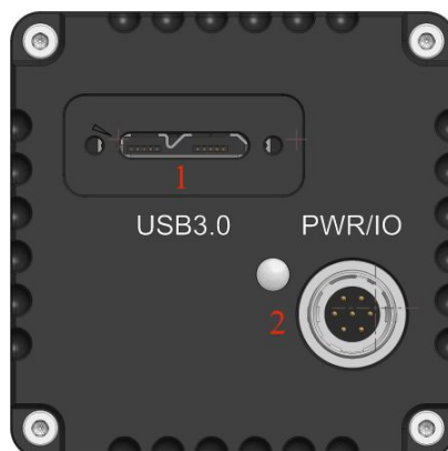
Figure 8- 19 USB interface small size camera
