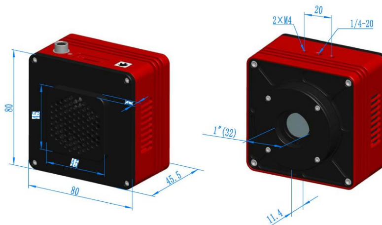
Figure 8- 1 USB interface refrigerated camera dimensions
