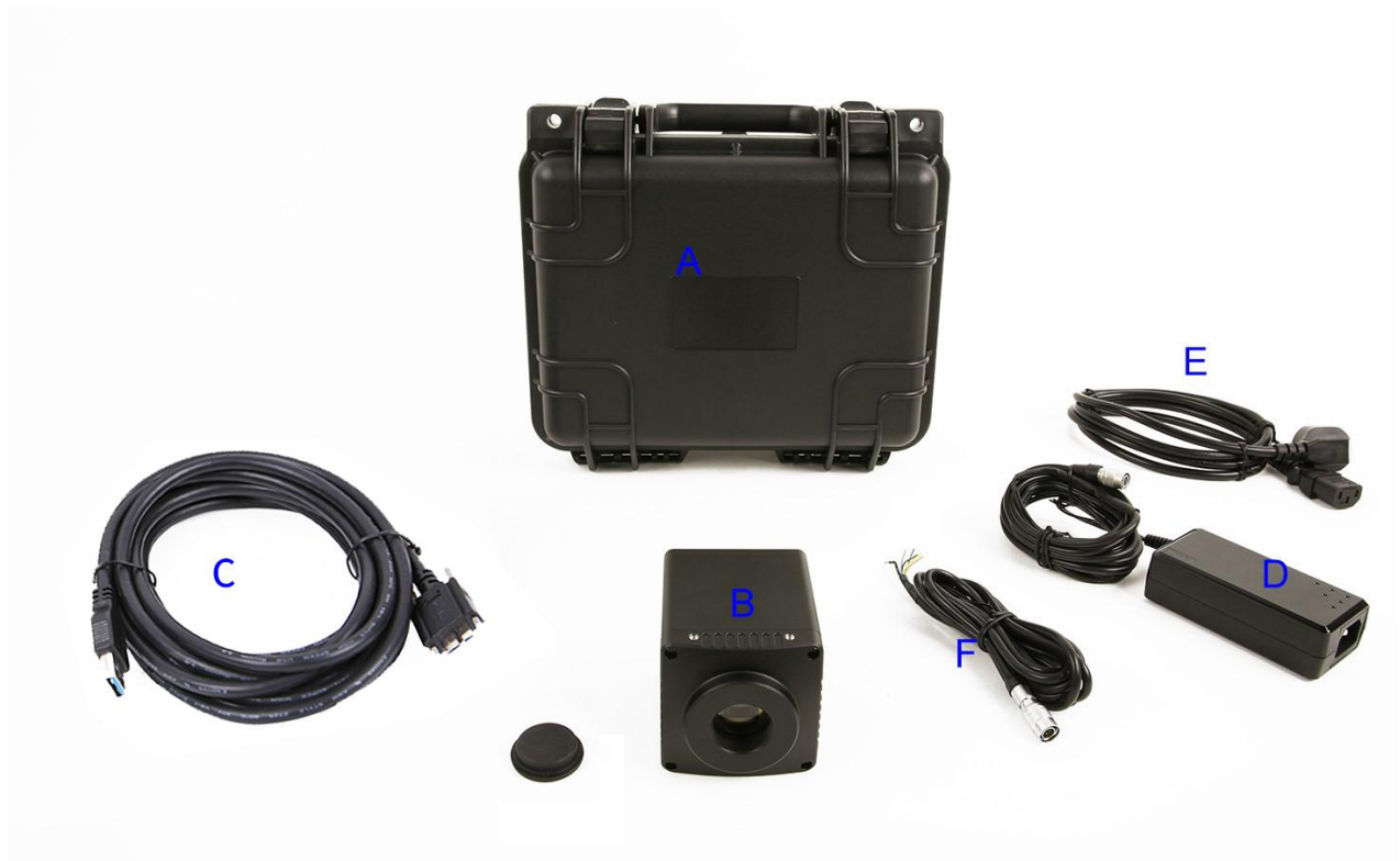
Figure 9- 7 USB camera packing information
