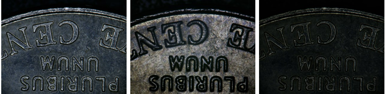
Figure 18 From left to right, there are three pictures of coins taken under left) LED Direct Ring Light Illumination; middle) LED Direct Ring Polarization Light Illumination; right) Coaxial Light Illumination
