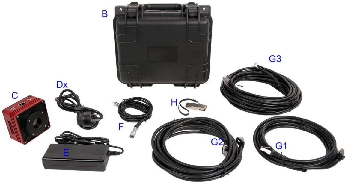
Figure 9-2 GigE refrigerated camera packing information
