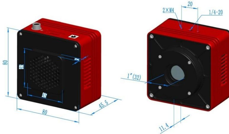
Figure 8-1 USB interface refrigerated camera dimensions
