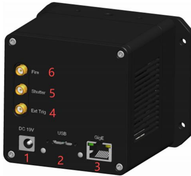
Figure 5-8 SC01AM-TE Camera interface diagram
